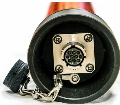
The new 100 Series Phoenix Induction Sensors eliminate the decades old artificial division of MT spectrum into combined Audio-Frequency MT (10 kHz to approx. 1 Hz) and MT (approx 400 Hz to 10,000 seconds).
